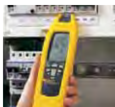
Location of fuses/breakers and assignment to circuits
